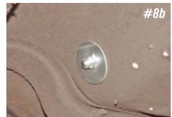
**Photo #8a & 8b:** The end of the seat belt is held to the driveshaft tunnel with a 1/2" X 1" bolt, a large and small washer and a lock nut.
