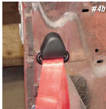
**Photo #4a & 4b:** The upper seat belt slide has a 7/16" X 1" bolt that passes through the inner quarter panel and bolts solid to the 1" X 2" bracket. Tighten the bolt and install the plastic cover. The cover can be painted to match the interior if so desired.
