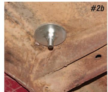
Photo #2a & 2b: The 7/16" bolt and small flat washer pass through the bracket and floorboard. Install the large flat washer and lock nut on the bottom side of the floor and tighten.
