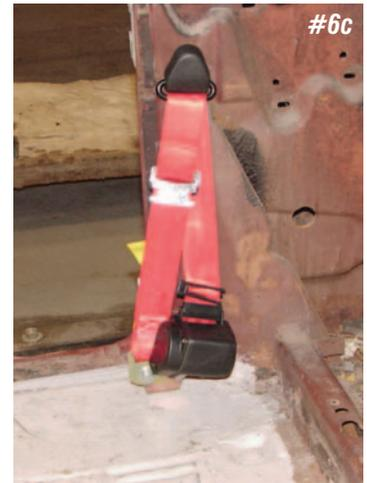
**Photo #6a, 6b & 6c:** The seat belt retractor and the end of the seat belt are held to the floor bracket with a 7/16" X 1" bolt with two flat washers and a lock nut. Mount the retractor to the rear hole on the bracket and the end of the seat belt to the forward hole.
