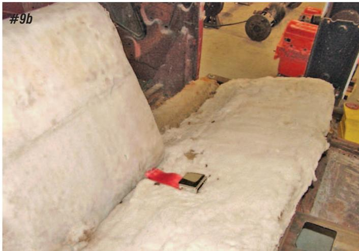
**Photo #9a & 9b:** The seat belt retractor keeps the long part of the seat belt gathered up and the clasp end will lie on the front seat neatly. The retractor has an internal clutch just like your late model car that will engage in the event of a sudden stop or crash.
