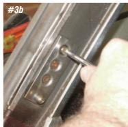
Photo #3a & 3b: The bracket on the liftgate installs with the pivot ball to the inside of the glass frame. The bracket on the body installs with the pivot ball to the bottom.
