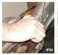
Photo #5a & 5b & 5c: With your hand (not a hammer!) push and snap the ends of the supports onto the pivot balls with the small piston rod end of the support attached to the bracket on the body. Once the sockets are connected to the balls, use your hand to push the retaining clip back in place.
