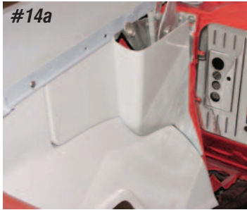
Photo #13 & Photo #14a & 14b: If an aftermarket A/C is installed on a 1957, the fresh air ducts will not be needed. This leaves a huge void around the hood hinge areas. To cover these areas a hinge cover is available to finish off
