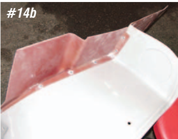
Photo #13 & Photo #14a & 14b: If an aftermarket A/C is installed on a 1957, the fresh air ducts will not be needed. This leaves a huge void around the hood hinge areas. To cover these areas a hinge cover is available to finish off
