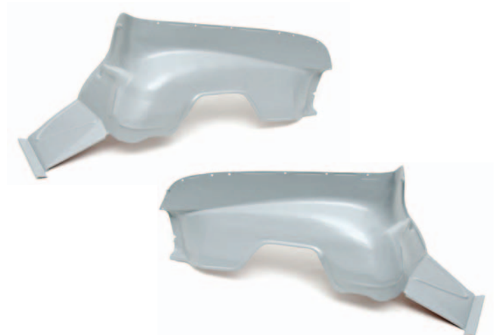
Photo #16: The custom fiberglass fender wells for the 1955 and '56 cars have also had all the holes removed and the factory reinforcement ribs deleted. In addition, the lower inner fender flaps are molded right in for an easy 1-piece installation. Good luck! ▽
