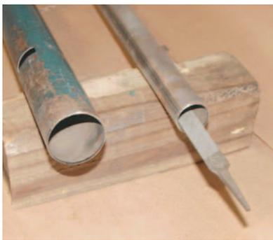
**Photo #4:** After cutting the shift tube and mast jacket, use a file and remove any burrs. The new bushing in the kit must fit true into the mast jacket and around the shift tube.
