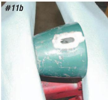
**Photo #11a & 11b:** Since this car has a floor shifter, the shift collar is fully inoperable. If you wish, you may remove the old shift handle boss from the collar and with a little body work it can be made to look like a shift lever was never there. Good luck!
