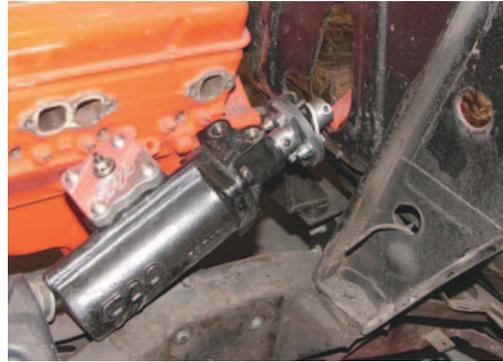
**Photo #1:** With the power steering box and coupler installed there is only about 1" of clearance between the coupler and firewall.
