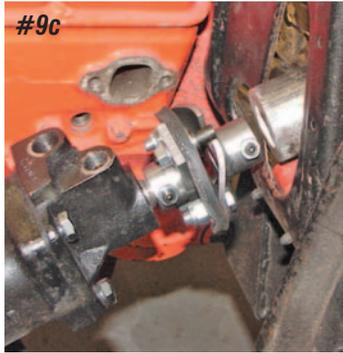
**Photo #9a & 9b & 9c:** The mast jacket will now be flush with the firewall. The stock mast jacket clamp that was bolted on the front side of the firewall will no longer work. **P/N 53-104** lower mast jacket clamp bolts to the inside of the firewall to hold the lower part of the mast jacket in place.
