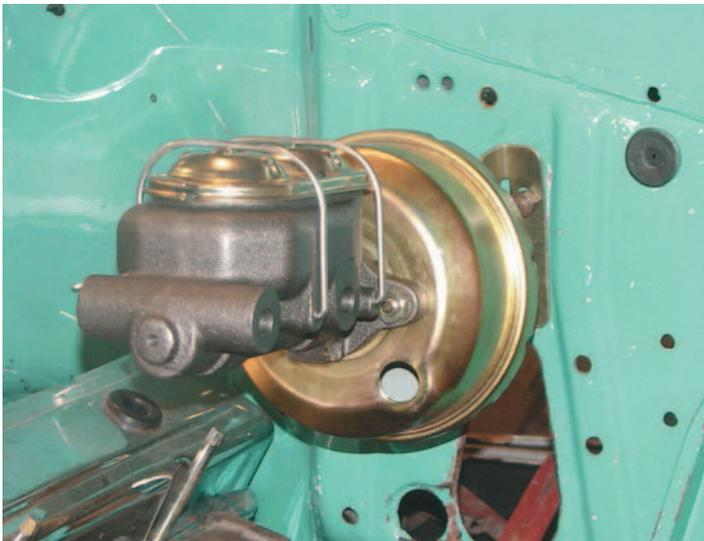
**Photo #1:** A dual master cylinder has two outlet ports. If an adjustable proportioning valve is going to be used, the front port of the master cylinder will be used for the front brakes and the rear port will be used for the rear brakes.
