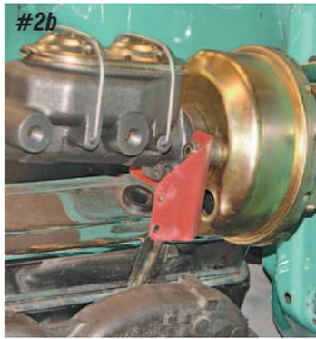
**Photo #2a & 2b:** The adjustable proportioning valve bracket **P/N 20-35** can be used with power brakes or manual brakes. The proportioning valve bracket is held in place with the two master cylinder mounting studs.
