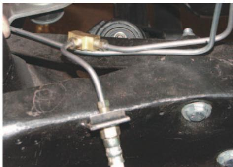
**Photo #9:** A 3/16" X 5" brake line is supplied to connect the 3/16" tee to the left front wheel.
