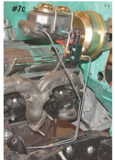
**Photo #7a & 7b & 7c:** A 3/16" X 24" brake line is supplied with a large fitting on one end and a small fitting on the other. This line is for the front brakes. The larger fitting screws into the front port of the master cylinder for the front brakes. The line is routed down to just behind the left upper control arm.
