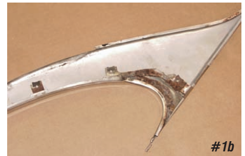
Photo #1a & 1b & 1c: The dogleg moldings are held to the body with three #6 button head sheet metal screws behind the sail panel. One #6 countersunk sheet metal screw at the front of the molding is trapped between the upper quarter glass stainless steel channel and the body with two #6 button head screws. In addition, the molding is attached to the body at the rear under the rear glass rubber via a rectangular metal tab that is screwed to the pinchweld.
