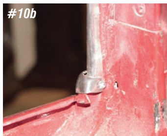
Photo #10a & 10b & 10c: The outer lower vent window stainless is held to the door with #6 counter sunk sheet metal screws included in kit P/N 34-38 . These moldings need to be installed before the vent window assemblies are installed. Good Luck. ✓
