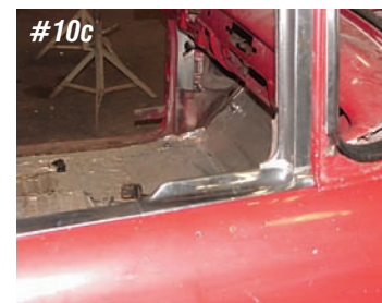
Photo #10a & 10b & 10c: The outer lower vent window stainless is held to the door with #6 counter sunk sheet metal screws included in kit P/N 34-38 . These moldings need to be installed before the vent window assemblies are installed. Good Luck. ✓
