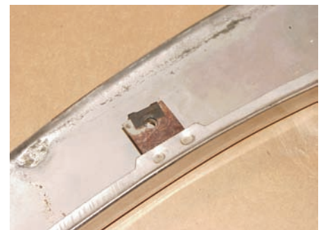
Photo #2: New J-clips are supplied with kit P/N 34-301 for the three tabs on the dogleg. These clips slide onto the tabs on the dogleg.
