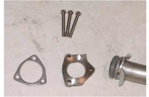
Photo #6: The passenger side exhaust manifold always uses a heat riser. A heat riser P/N 24-01 or heat riser delete P/N 24-03 must be used to properly space the exhaust pipe so it will line up with the rest of the exhaust system.
