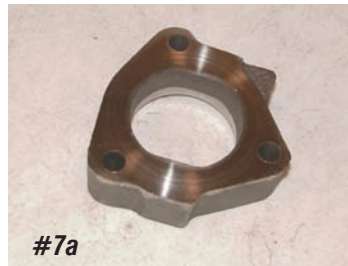
Photo #7a & 7b: The heat riser or heat riser delete is flat on one side and concave on the other. The flat side fits the exhaust manifold and the concave side fits the exhaust pipe donut.
