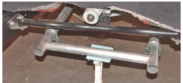
Photo #9: Next, install the H-pipe. The front of the H-pipe will slip up over the exhaust pipes and is held to the exhaust pipes with a muffler clamp. This fully functional H-pipe improves horsepower by equalizing the exhaust pulses as close to the engine as possible.
