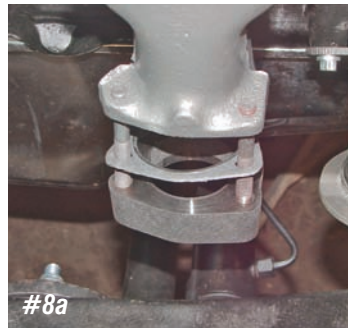
Photo #8a & 8b: The flat gasket included with the exhaust system seals the heat riser or heat riser delete to the exhaust manifold. With the heat riser or heat riser delete in place, install the passenger side exhaust pipe leaving the three nuts loose at this time.
