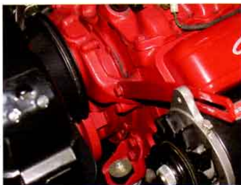
Photo #3: The upper adjusting arm for the generator attaches to the upper water pump bolt and has a slot where the belt tension is set off an ear on the generator case. The stock generator adjusting arm will be deleted so remove the
