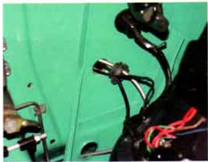
Photo #16a & 16b: The new harness can be passed through the firewall using one of the holes in the speedometer cable grommet. Remove the grommet and place the wire in one of the holes and then install the grommet back into the firewall.
