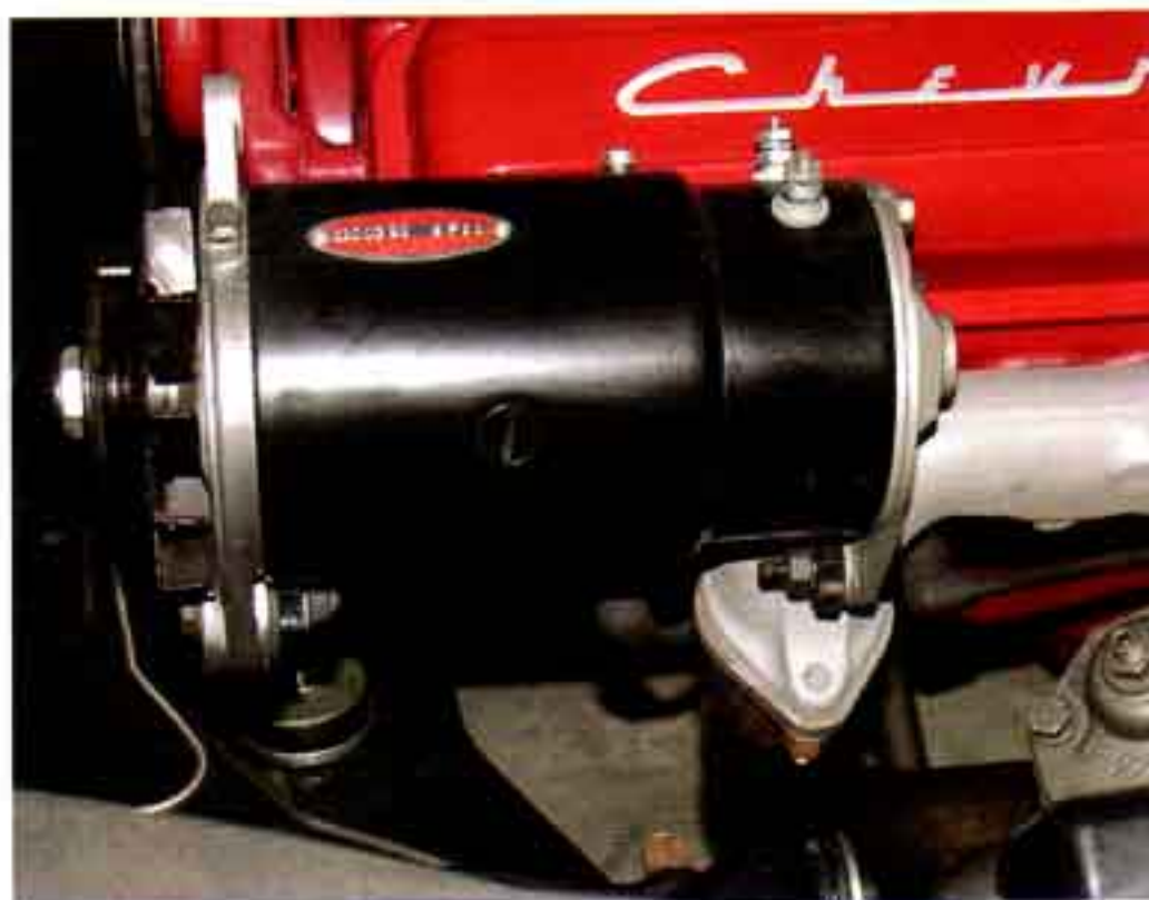
Photo #4: The generator has two lower ears that mount to a bracket that is bolted to the exhaust manifold. Each ear has a 5/16" X 1-1/2" bolt.
