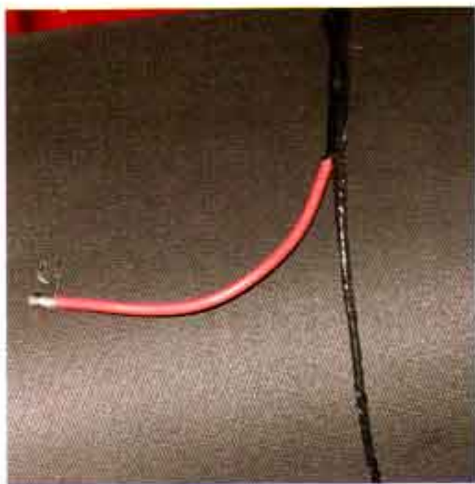
Photo #15: There is a large red wire with a 90 degree fork connector that will connect to the battery terminal lug on the horn relay. We are going to leave the stock voltage regulator in place so the wires can stay connected to the voltage regulator but if you want, the wires can be tapped up into the harness and be hidden.
