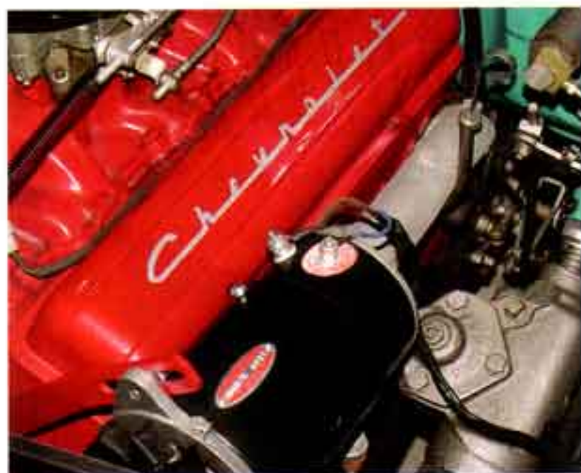
Photo #2: The generator is mounted on the drivers side of the car rather if the car has a 6 cylinder or V-8 engine. The generator has two wires connected to the top rear of the case with a nut and lock washer, both these wires will need to be disconnected.
