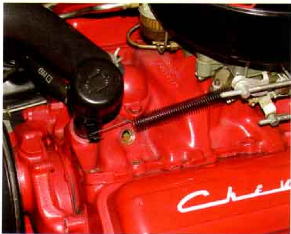
Photo #7a & 7b: The water temperature sender has 1/2" pipe threads and screws into the intake manifold just over the second intake bolt on the drivers side, with pipe thread the sender may be very tight so a 1/2" breaker bar and a 6-point socket is always a good idea to use when removing a temperature sender.
