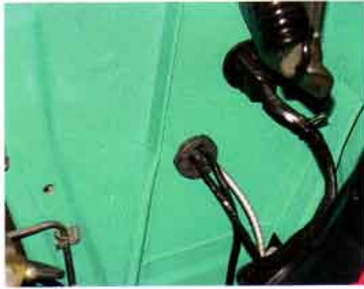
Photo #16a & 16b: The new harness can be passed through the firewall using one of the holes in the speedometer cable grommet. Remove the grommet and place the wire in one of the holes and then install the grommet back into the firewall.
