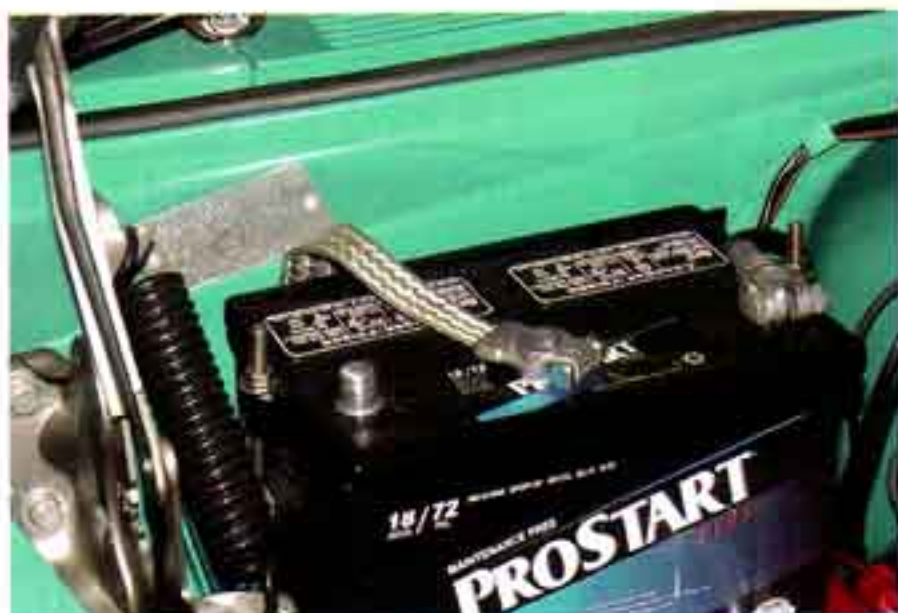
Photo #1: The first thing to do when ever working on the electrical system on a car is to disconnect the negative battery cable.
