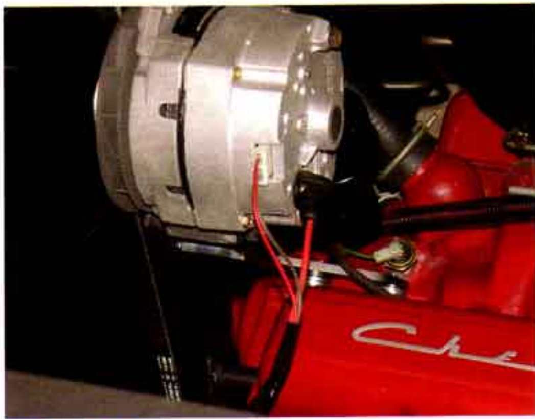
Photo #14: The adapter harness has a large red wire with a black boot that will connect to the 1/4" stud on the back of the alternator. The adapter harness also has a two pin connector that will plug into the side of the alternator also.
