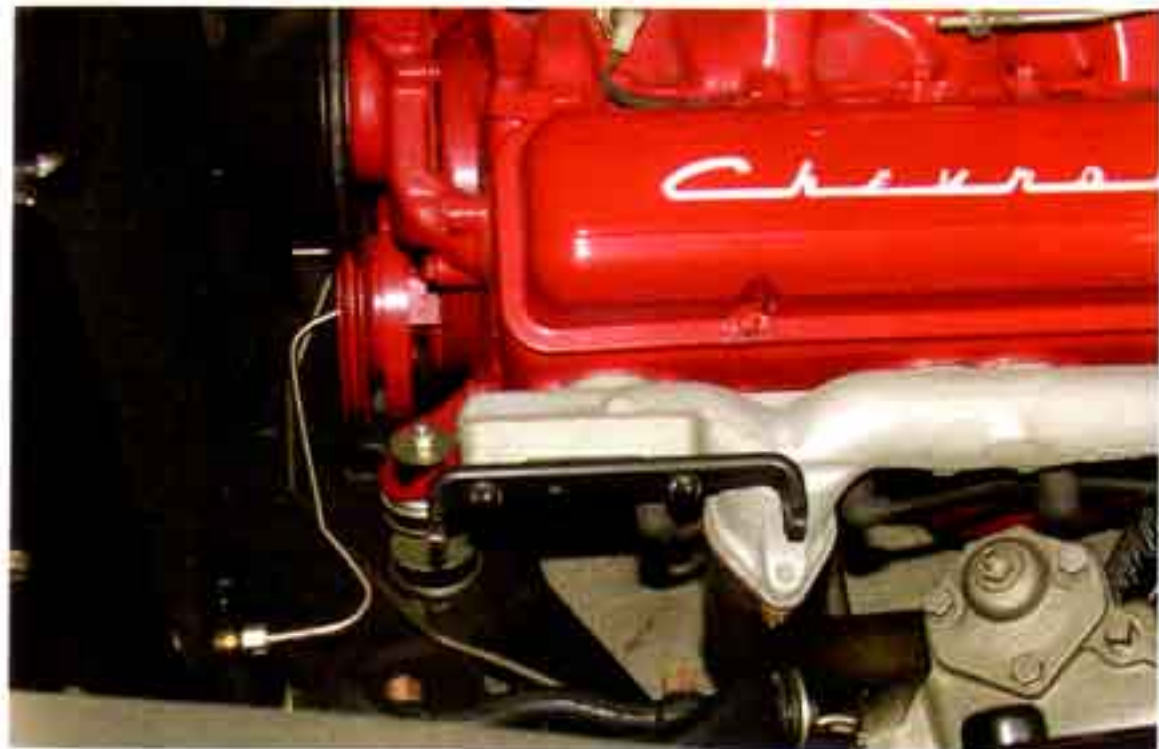
Photo #5: The lower generator bracket is bolted to the exhaust manifold with two 3/8" X 1" bolts and lock washers, it is a good idea to use some penetrating spray on these bolts if they have been in for a while.
