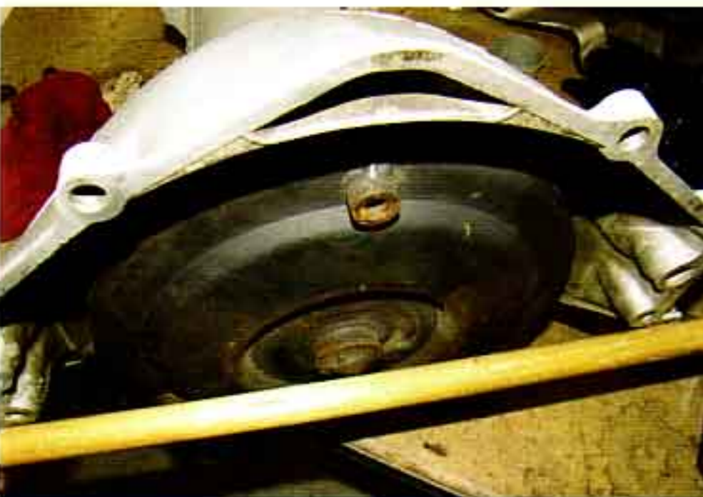
bolting to the back of the engine, damage will occur to the front pump of the transmission. To make sure the converter is in all the way, lay a straight edge on the bellhousing. The snout on the converter should be flush with the straight edge.
