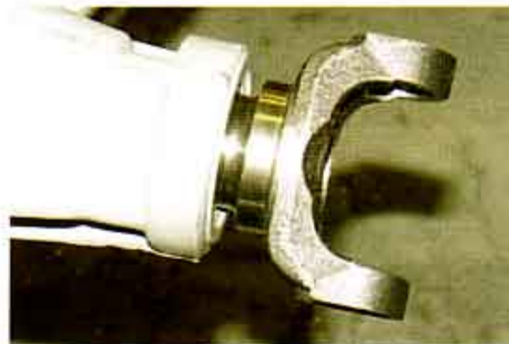
Photo #27a & 27b: The driveshaft yoke P/N 19-36 is the same as a TH350 and TH700-R4. Install the yoke into the tail shaft of the transmission and push it in until it bottoms out. Now pull the yoke out 1" and measure from the center of the front cup to the center of the rear cup on the rear end and have your driveshaft shortened appropriately at a driveline shop.
