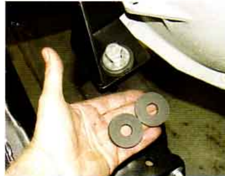
Photo #8a & 8b: The upper and lower brackets are held together with a 1/2" X 2" bolt with flat washers, a castellated nut and cotter pin. Tighten the nut and install the cotter pin so that there is a slight squeeze on the rubber grommets. This will insulate any engine vibrations from the frame and body.
