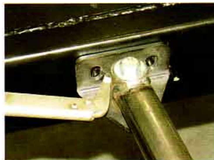
Photo #14a & 14b: Square the crossmember in the frame and using a C-clamp, hold the left and right elbow brackets in place. Drill an 1/8" pilot hole into the frame centered in the elbow mount bracket holes.
