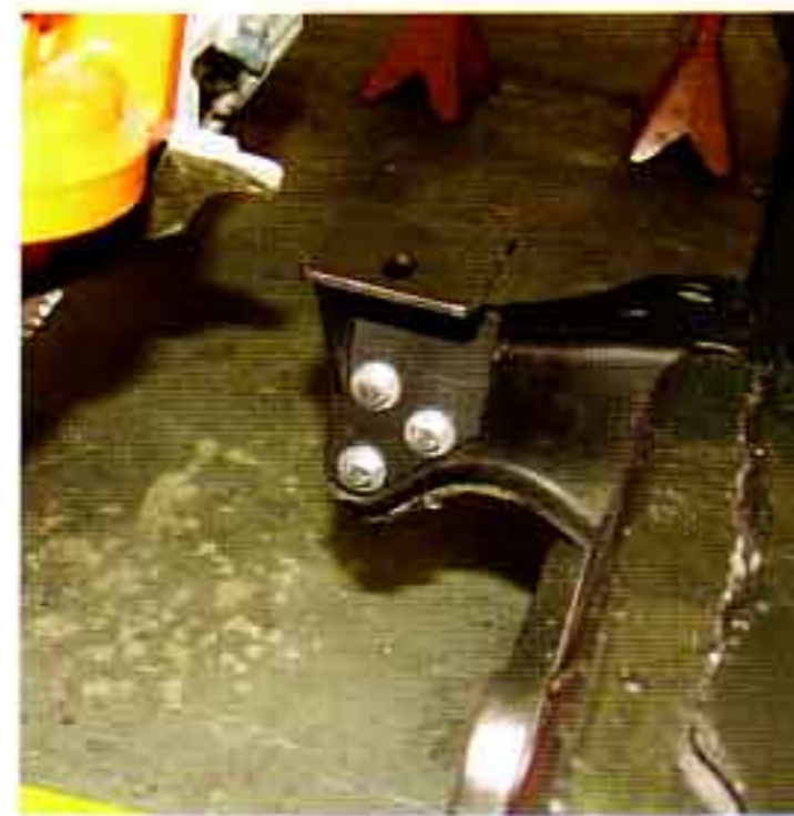
Photo #6a & 6b: The lower half of the new transmission supports bolt to the front of the original frame horns with three 3/8" X 3-1/4" bolts, flat washers, lock washers and nuts. There is a cut-out on the drivers side lower bracket to allow the front emergency brake cable to pass by.
