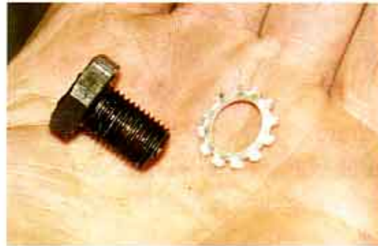
Photo #3: The flywheel is held to the crankshaft with five 7/16" X 11/16" fine thread bolts with serrated lock washers P/N 19-62. Torque these bolts to 45 ft/lbs.
