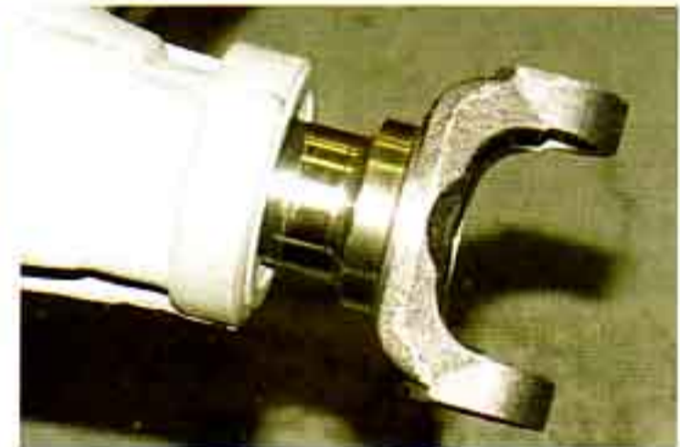
Photo #27a & 27b: The driveshaft yoke P/N 19-36 is the same as a TH350 and TH700-R4. Install the yoke into the tail shaft of the transmission and push it in until it bottoms out. Now pull the yoke out 1" and measure from the center of the front cup to the center of the rear cup on the rear end and have your driveshaft shortened appropriately at a driveline shop.
