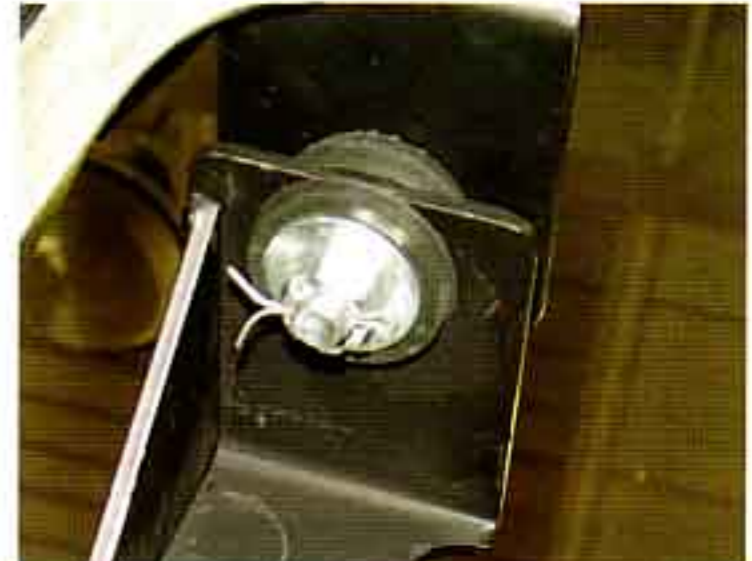
Photo #8a & 8b: The upper and lower brackets are held together with a 1/2" X 2" bolt with flat washers, a castellated nut and cotter pin. Tighten the nut and install the cotter pin so that there is a slight squeeze on the rubber grommets. This will insulate any engine vibrations from the frame and body.
