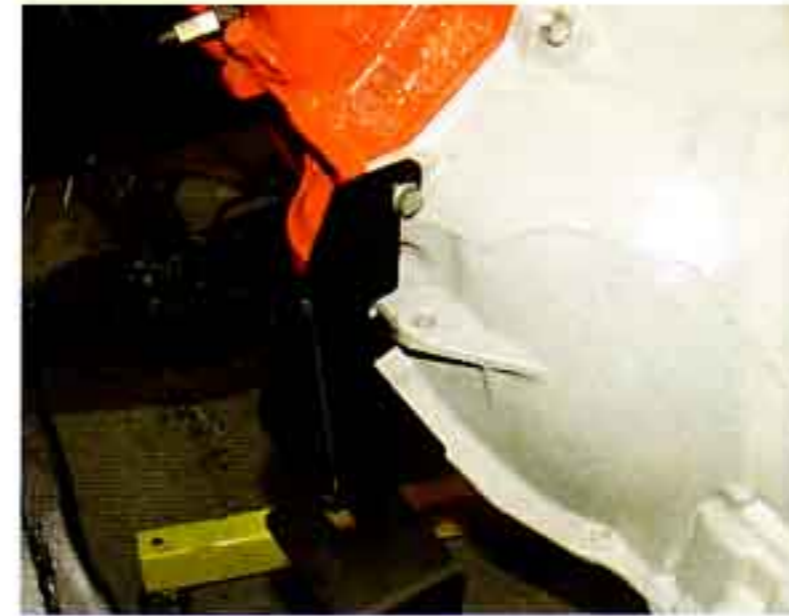
Photo #6a & 6b: The lower half of the new transmission supports bolt to the front of the original frame horns with three 3/8" X 3-1/4" bolts, flat washers, lock washers and nuts. There is a cut-out on the drivers side lower bracket to allow the front emergency brake cable to pass by.
