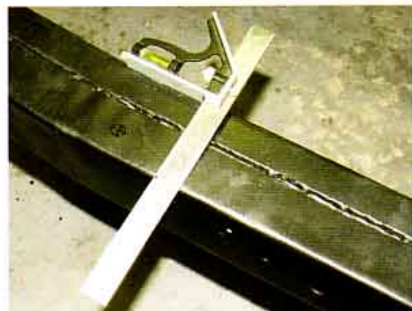
Photo #15: Remove the crossmember and elbow mounting brackets. Using a square, mark the outside of the frame and drill all four 3/8" elbow mounting bracket holes.
