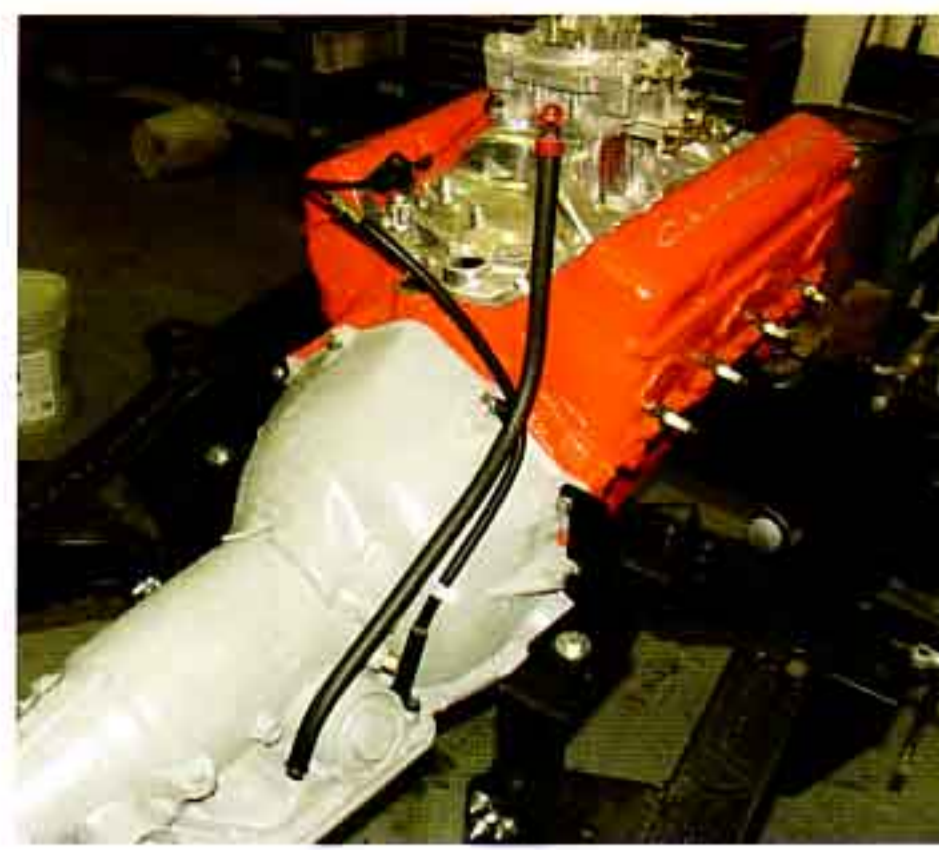
Photo #25: The dipstick and tube P/N 19-166 is held in place using the right hand upper bellhousing bolt.
