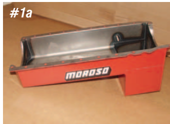
Photo #1a & 1b: The oil pan is a rear sump design and holds 6 quarts of oil including the oil filter.
