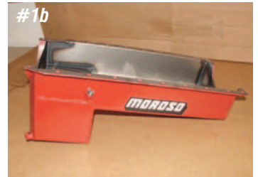
Photo #1a & 1b: The oil pan is a rear sump design and holds 6 quarts of oil including the oil filter.
