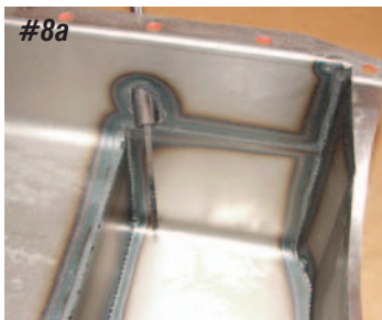
Photo #8a & 8b: The dipstick will protrude out the bottom of the dipstick tube into the sump of the oil pan. Fill the engine with six quarts and
