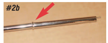
Photo #2a & 2b: Most GM and some aftermarket big block oil pans have a female fitting in the side of the oil pan for the dipstick tube. The dipstick tube has a ring 4" from the bottom. When the dipstick tube is installed in the oil pan the ring will fit tight in the female fitting.
