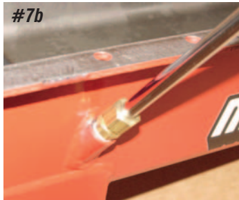
Photo #7a & 7b & 7c: Install the dip stick tube into the fitting in the oil pan making sure the tube bottoms out in the fitting. With a wrench holding the fitting in the oil pan, tighten the nut on the dipstick tube.
