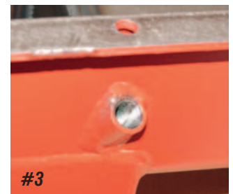
Photo #3: The Classic Chevy Moroso oil pans utilize a 1/4" pipe bung welded into the side of the oil pan to receive the dipstick tube. This is far superior way to connect the dipstick tube to the oil pan with no chance of leaks.
