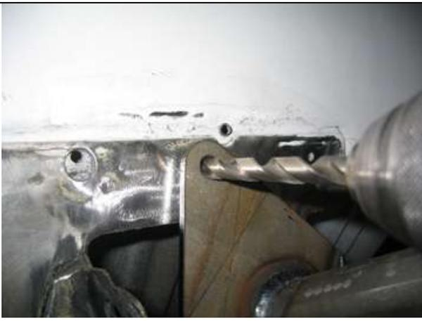
**Drill 3/8 hole through the firewall using the mounting bracket as a guide.
