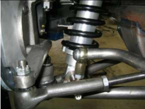
Complete installation by fastening the upper 1/2 inch rod end of the sway bar link from the lower shock mount bolt to the end of the anti-roll bar with the 1/2-20 x 1 1/2 inch button head bolt.
