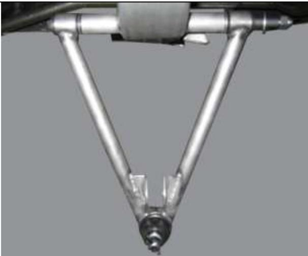
**Continue with the front suspension component installation. First, install the lower control a-arm shaft with acorn nut towards the front of the car into lower A-arm (shock mounting tabs facing up) and through the cross-member, the washers go on each side of the bushings.**
