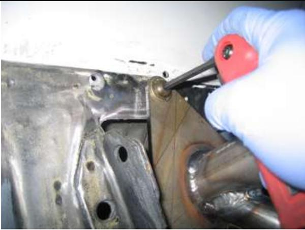
**Then fasten it with the supplied 3/8-24 X1 Button Head Bolt**
