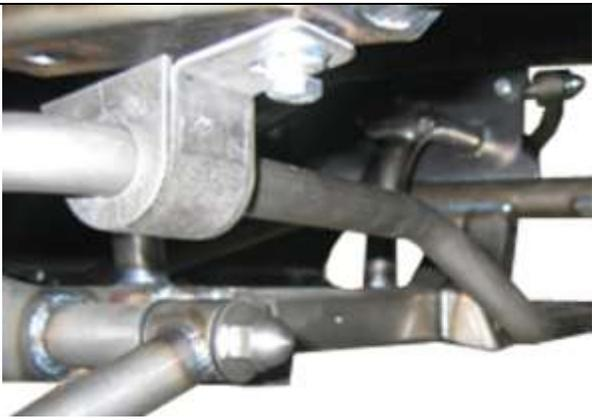
Install the front anti-roll bar into position using the supplied polyurethane and saddle mount making sure that the stepped down center section is down to clear the engine pulley. Fasten anti-roll bar saddle mount using the supplied 3/8-16 x 1 inch hex head bolt; 3/8 inch lock and flat washer.
