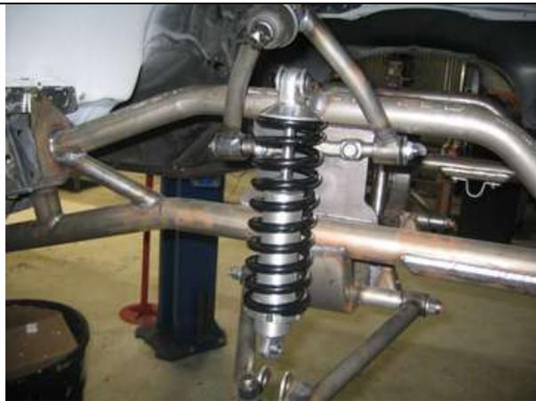
**Install the shock to the upper mount using the supplied ½ -20 by 1 ¾ inch button head bolt and ½ -20 half height nut.**
