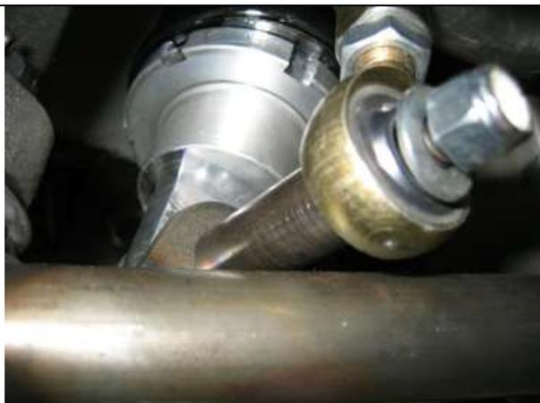
**Next, install the shock into the lower a-arm tabs making sure that the adjustment dial towards the rear of the vehicle and install the 3 ¾ inch shoulder bolt from the rear through the rear bracket, then the shock bearing, front bracket, then the spacer and last the rod end link for the sway bar. Install the washer and nut and tighten. The top rod end will be attached to the sway bar later.**
