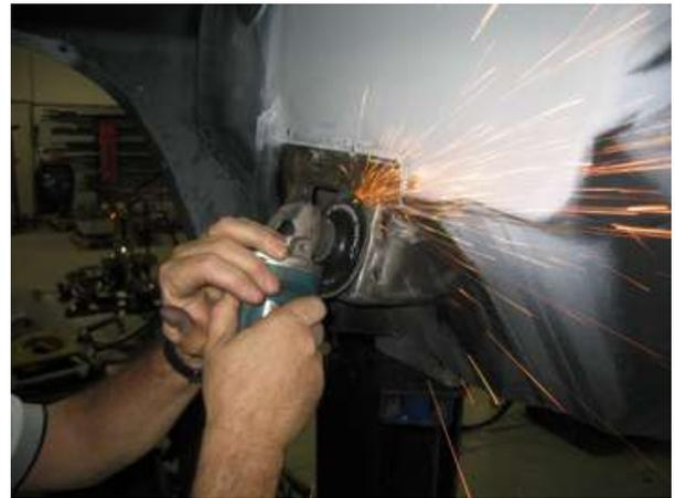
**Prep the firewall mounting surface edge on the firewall side by grinding smooth the flange edge so that the clip will be mounted flush to the firewall.**
