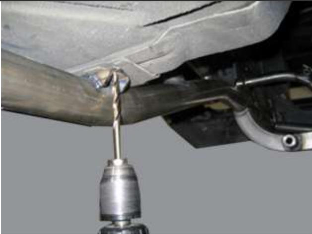
**Next, drill (2 holes per side) through the floorboard located between the firewall mounting point and the rear-most mounting point using a 5/16" drill bit.**
