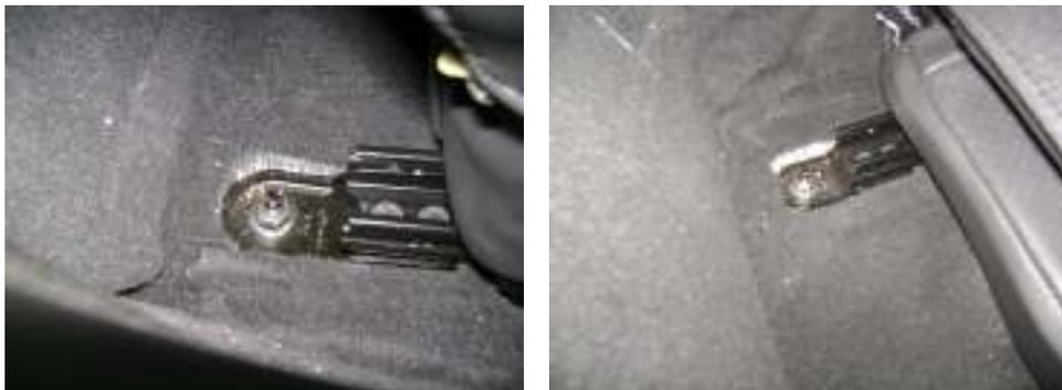
**STEP #3:** Remove the 15mm seat belt bolt. Do this by slightly lifting, and tilting the seat toward the center console tunnel to gain access to the seat belt bolt.
