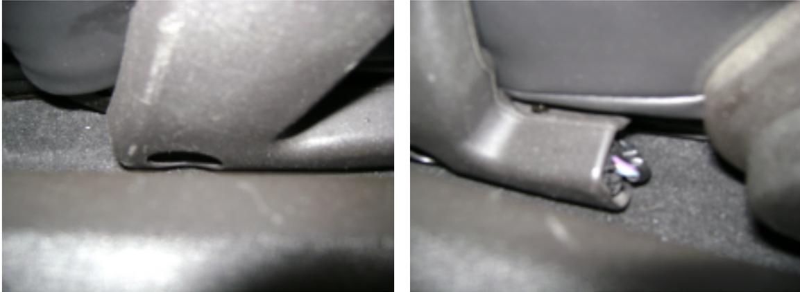
**STEP #4:** Tilt the seat back forward, then tilt the entire seat toward the rear of the car (leaving the seat back locked in the tilted forward position). This allows you to gain access to the plug under the seat.
