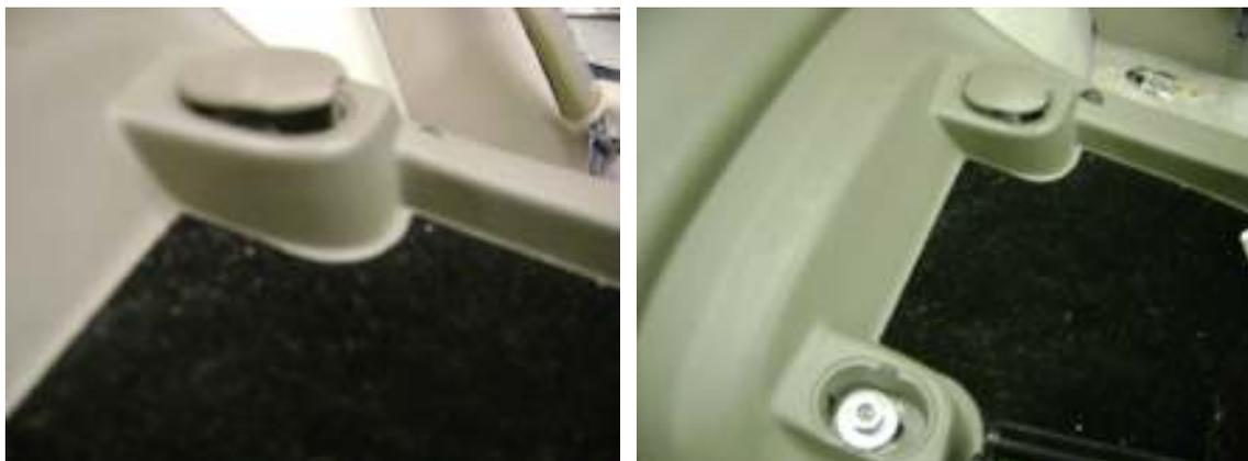
The console can now be moved back towards the rear of the car, and up, but the fuel door release is still hooked up. Remove the plug after positioning the console in a way that makes it easier for you to do so.
