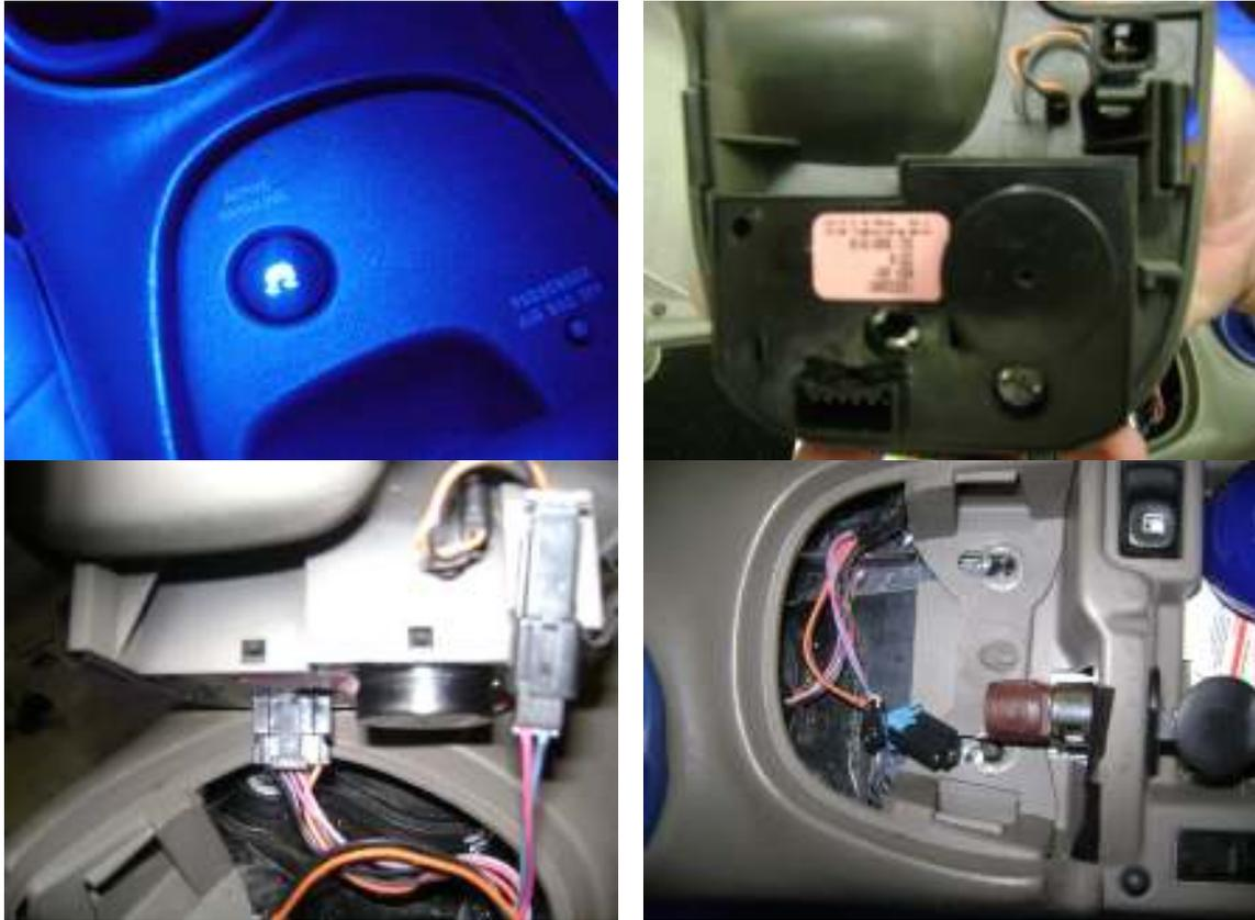
There are another (2) 10mm nuts that need to be removed at the rear of the console as well. Pop off the covers, and remove the nuts.
