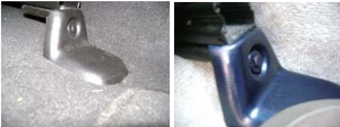
STEP #1: Remove seat bolt covers by pulling the center pin out, and then removing the clip on the cover.
