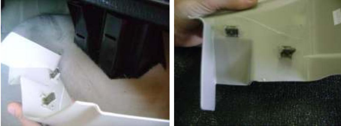
For the Verts, remove the rear speaker panel and the clips shown below need to be removed.
