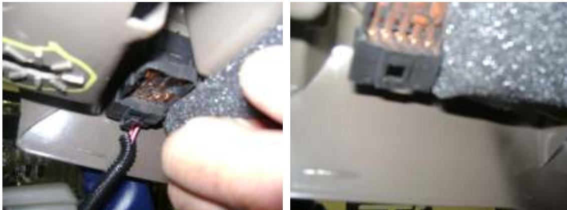
Now, you can remove the center console out of the car, and at the same time, gently start to lift up on the dash bezel, and do so GENTLY, so as not to break the upper tabs show below.
