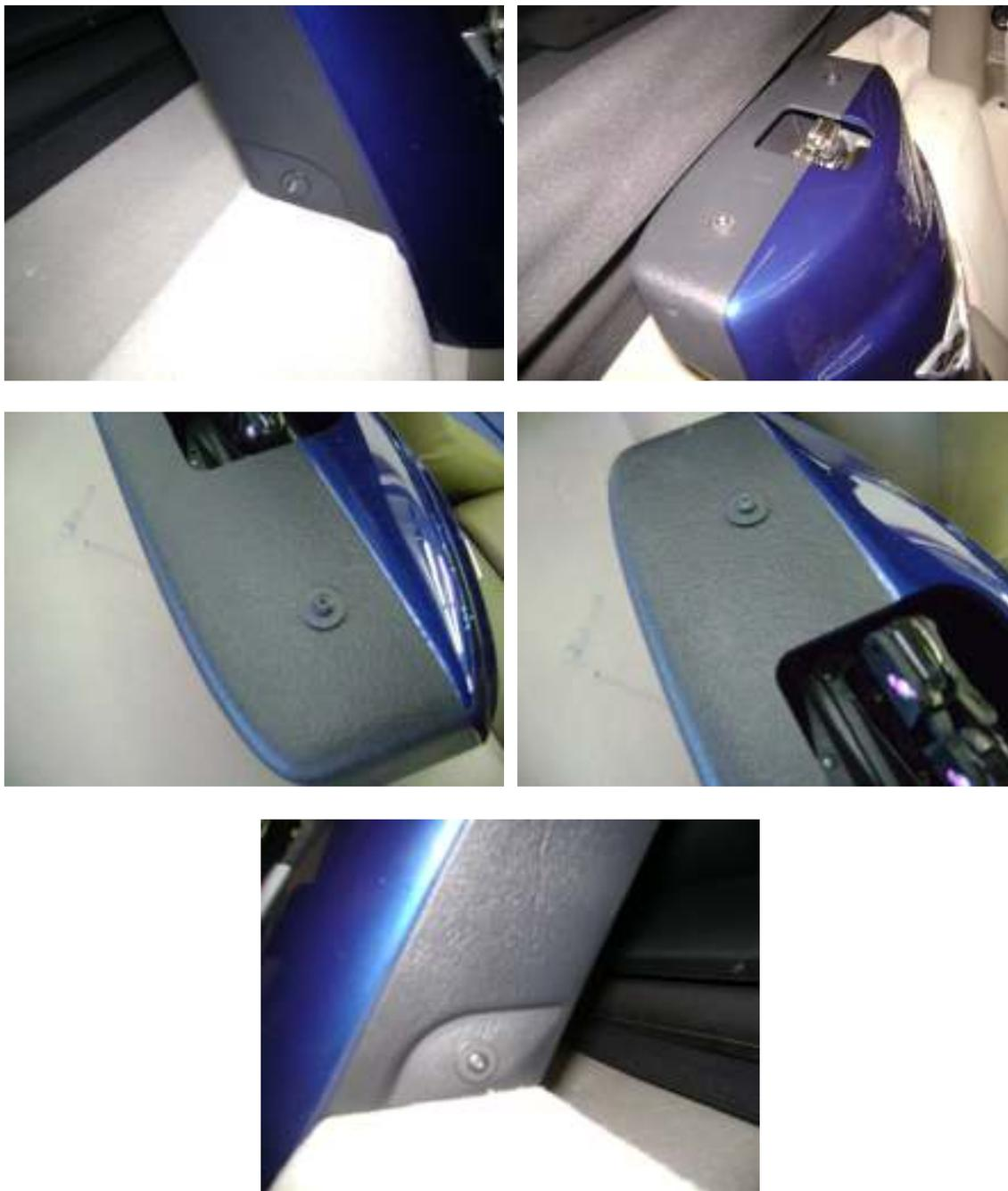
After removing the screws, gently pull the waterfall up and place it in an area where it won't be scratched or damaged. You need to remove one of the brackets that hold the waterfall in order to remove the carpet.
