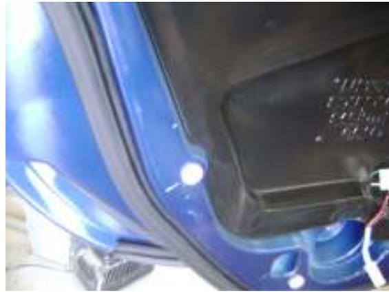
Once the clips are released, pull up on the door panel, releasing the metal clips that hook to the door just below the door window seal. See the picture below.
